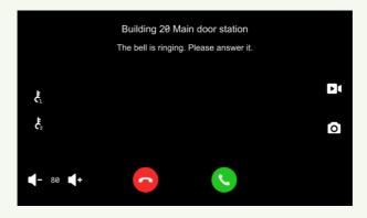
When someone makes a call via the door station, you can answer or hang up through the button shown on the screen. Meanwhile, you can adjust the call volume and enable mute as needed on the screen. In addition, you can open the door by tapping the unlock button as needed.
